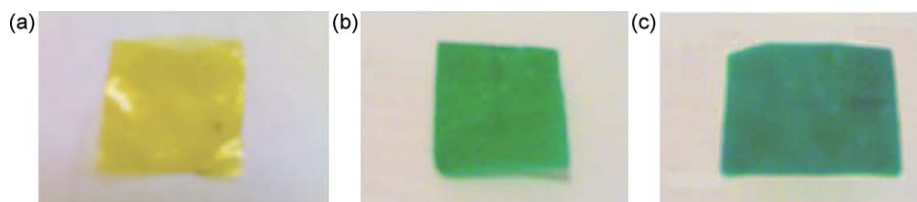
Fig. 5. Digital photograph of chitosan-ACHCA membranes after dipped into Coomassie Brilliant Blue solution of 5 ml for 5 min: (a) CACN-5 without lipase, (b) CACN-2 with lipase and (c) CACN-5 with lipase.
